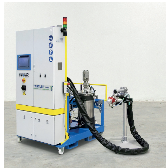
The Nodopur synthetic resin processing system: with automatically controlled mixing ratios and outputs of 0.1 to 100 l/min, it meters and mixes one or more components with viscosities from 1.0 to 60,000 mPas.
