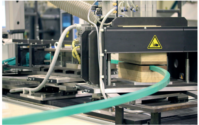
The result of pultrusion is a lightweight but highly resilient profile and molded part made of GRP or CFRP. © PulNet
